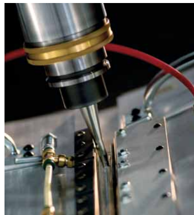
Laser beam welding is an alternative to friction stir welding
