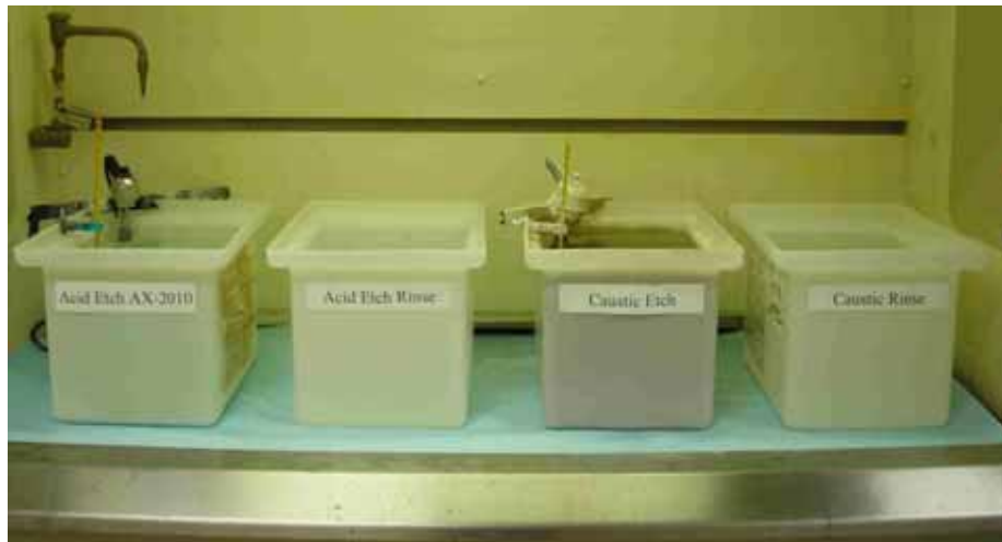
Figure 2. Houghton Metal Finishing, 20-L Pilot Line
