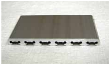
Figure 1. T-Slot Die Used to Promote Streaking
